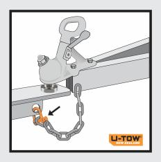
Connect the safety chain/s with D-Shackle/s to the towing vehicle. Cross over chains (if more than one chain) and do not allow to drag on the road.
