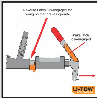
To release handbrake pull handle back and lift ratchet lever (if lever is included) away from locking grooves. NB: the ratchet lever must be in this position whilst towing trailer with vehicle.
