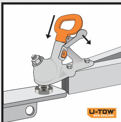
**Push handle down and release coupling handle trigger once positioned securely on tow ball. Coupling is now in the locked down position ready for towing.**
