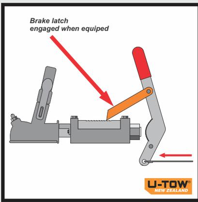
The handbrake is engaged when the handle is pulled back fully and ratchet lever is down in locking grooves (the ratchet lever is not fitted to all trailers). NB: wheel chocks MUST always be used also.
