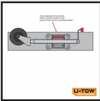
**Jockey Wheel/Stand MUST be in the horizontal position with both wheel and handle placed upwards before you commence towing.**
