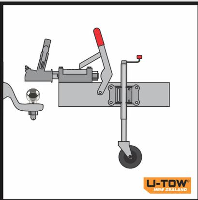
**Raise trailer with jockey wheel/stand to just above tow ball height and reverse vehicle to trailer (do not drag trailer to vehicle.)**
