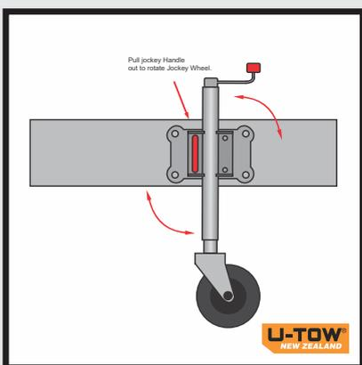
Pull out handle and rotate to enable Jockey Wheel/Stand to be put in the horizontal position (ensure no load/weight is on the stand).
