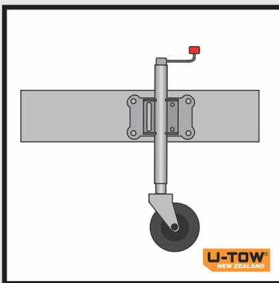
Jockey Wheel/Stand only to be in the vertical position when the trailer is being attached or unattached from the towing vehicle, or in a parked position.
