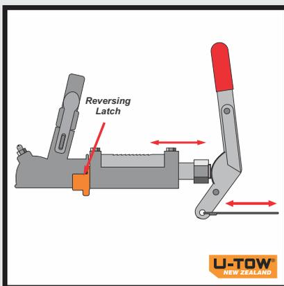
The trailers brakes are operational when the reverse latch is in the OPEN position.
